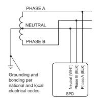
Figure 3-3. Split Phase Wiring Diagram
